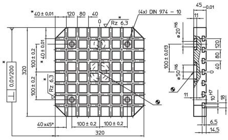
$<sup>^{\</sup>star}$  These tolerances are valid only for optional exterior stop type. Slot spacing 40 ±0,01.
